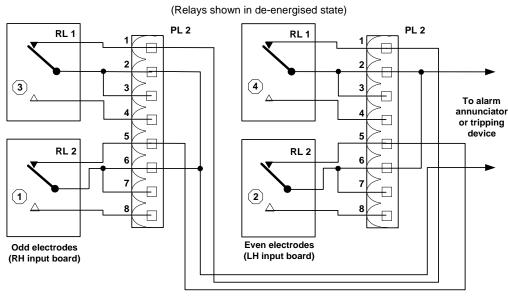
Case A - Relays normally energised, de-energise one in each pair to trip
